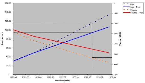
Fig. 21: Changes in area capacity due to hydrological intervention
