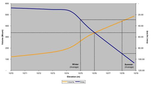
Fig 8 : Area Capacity curve for Wular Lake
