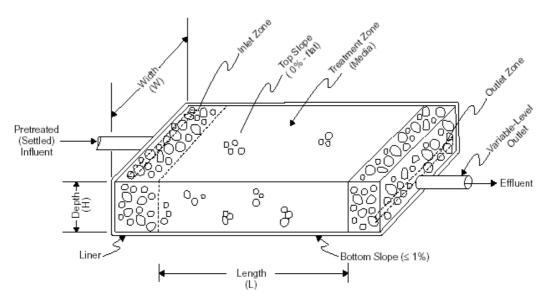
Fig. 4.2 Cross-section design of Constructed Wetland compartment
