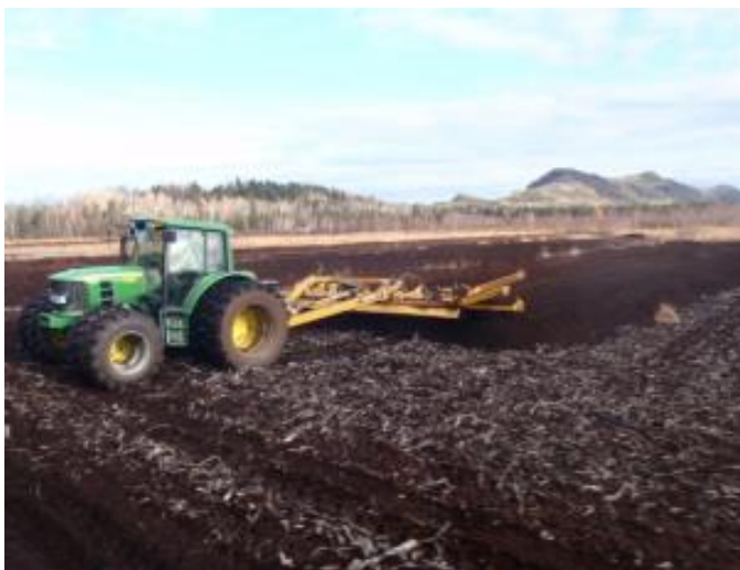
Figure 5.7. In Canada, large scale restoration is performed with widely-used agricultural machinery. To allow the circulation of heavy machinery and avoid creating ruts, the first steps of restoration (site preparation, plant, straw and fertilizer spreading) are performed on drained peat and rewetting is carried out right after the previous operations are over. Restoration operations can be performed on a rewetted site when the ground is frozen. Restoration sites are prepared and levelled with a leveler or a bulldozer. Plant material can be harvested with a rotovator or with a bulldozer (when moss carpet is frozen) and is then picked up and transported to the restoration area.
