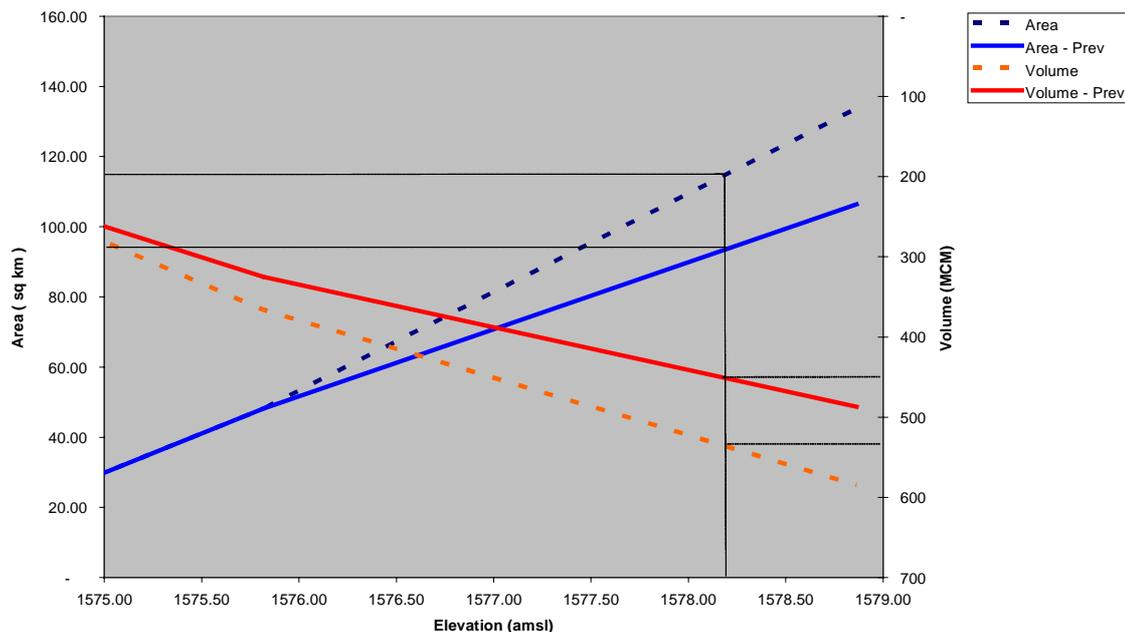
Fig. 21: Changes in area capacity due to hydrological intervention
